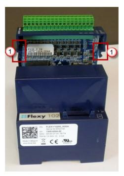
1 Hooks to be pressed are off-centered – press while pulling upwards
