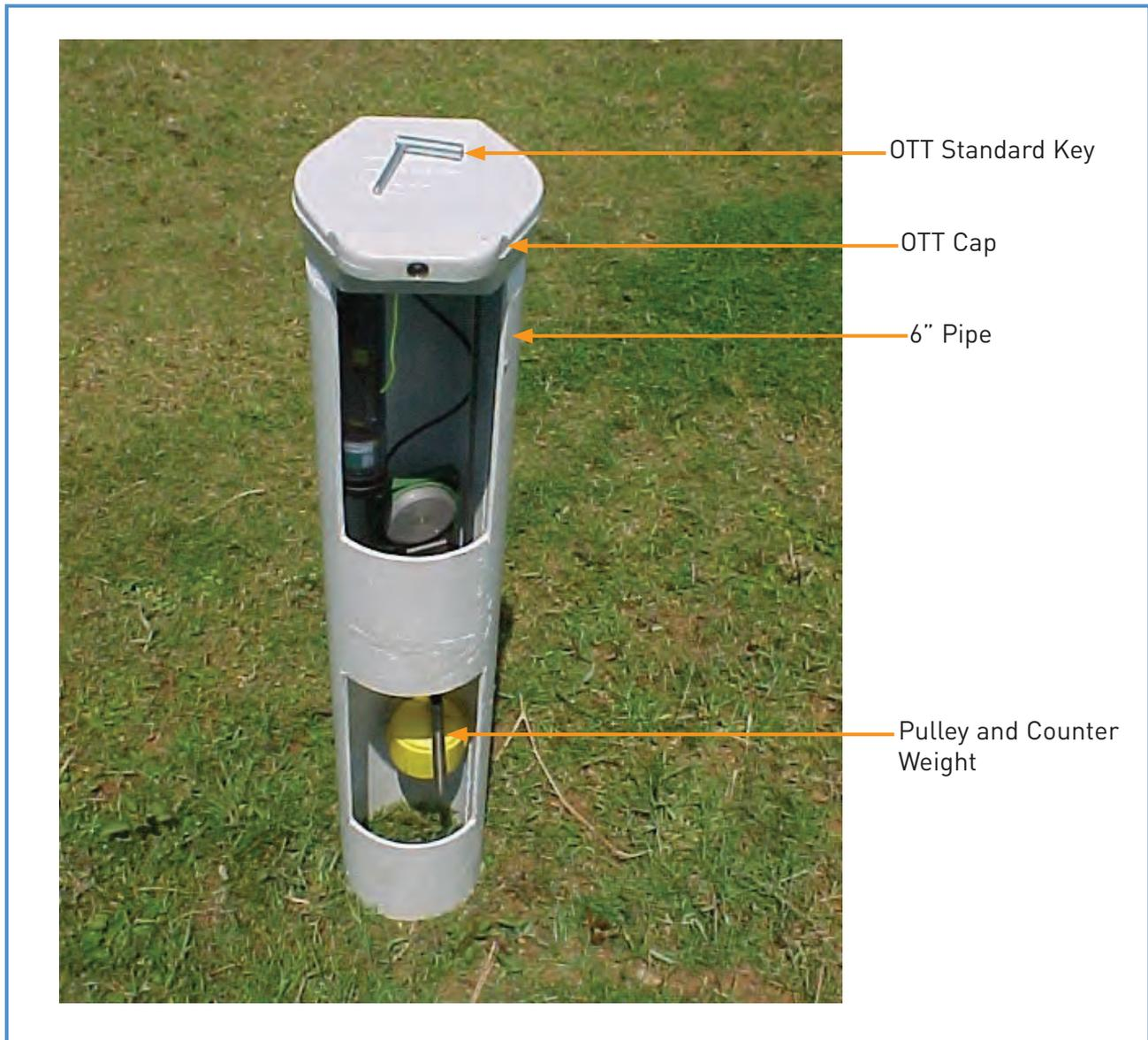
Figure 10: Thalimedes installed in a 6" demonstration pipe.
